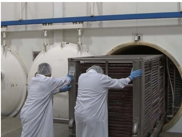
Placed in a refrigerated vacuum system, frozen raw materials are dehydrated without thawing. Thus, the ice in the product is sublimated into vapour.
