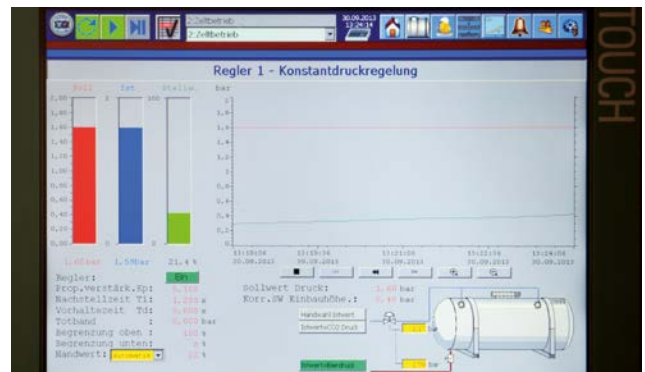
Fig. 3 The red actual line shows perfectly constant maintenance of the beer pressure at 1.6 bar. The setpoint line is hiding behind the actual line. The resolution of the display is adapted to the new conditions in the display.
