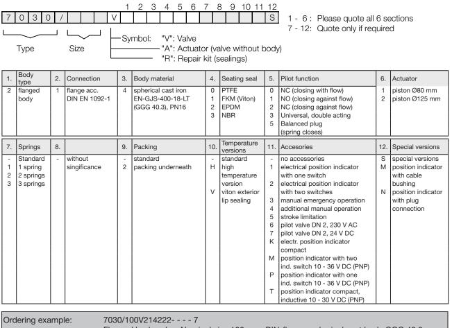
Flanged body valve, Nominal size 100 mm, DIN-flange, spherical cast body GGG 40.3, EPDM seat material, NC (closing against flow), piston 125 mm, pilot valve 24 V DC.
